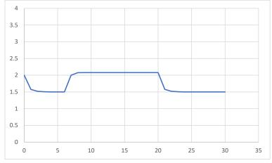
The error is in this case defined so that a level higher than the desired one (the set point value) results in a positive value. Thus the higher the value of the error, the higher the value of u(t) = Kv(t). (the resistance coefficient in the denominator means that this must be lower, ergo a larger opening)
