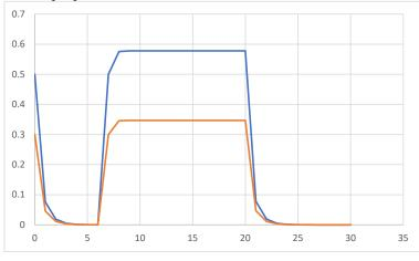
The plot below shows  $e(t) = h(t) - h_{sp}$  (blue) and u(t) = Kv (orange) vs. t. They have the same shape, i.e. are proportional to one another:
