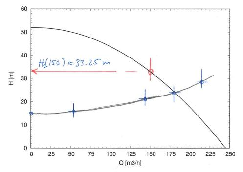
c) For the pump to deliver exactly 150 m3/h, a system head corresponding to the pump head at that rate is required. This can be read of the pump diagram; Hs (150 m3/h)  $\approx$  33.25 m.
